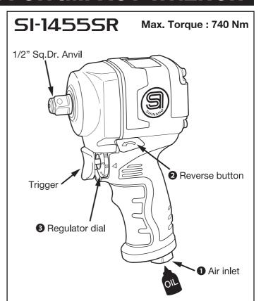
5. Prior to start the real operation, adjust the regulator dial 3 to scale numbers for torque adjustment.
